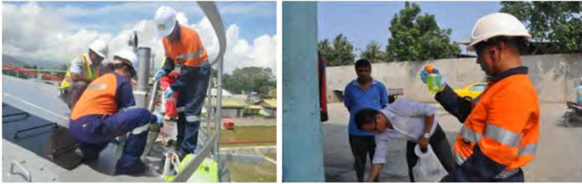
FIGURE 16: FUEL SAMPLING AT PERTAMINA STORAGE FACILITY & RUVIC FFS
