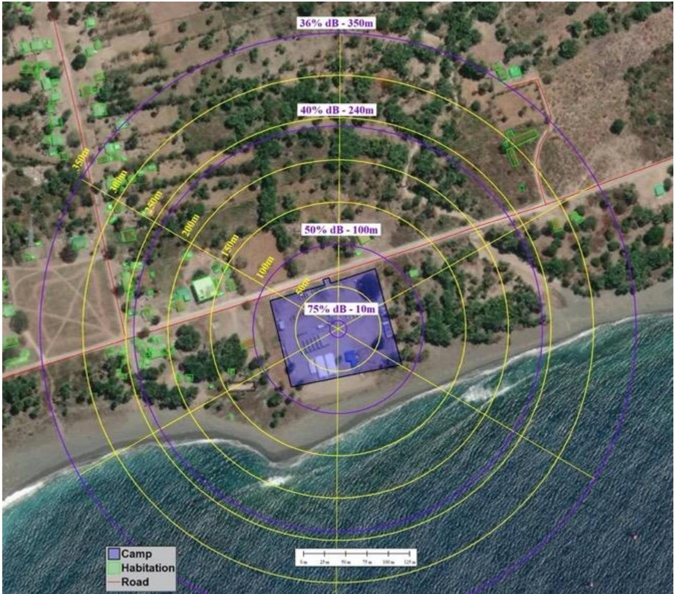
Figure 2-2 - Sound Attenuation at the Betano Base Camp Location
